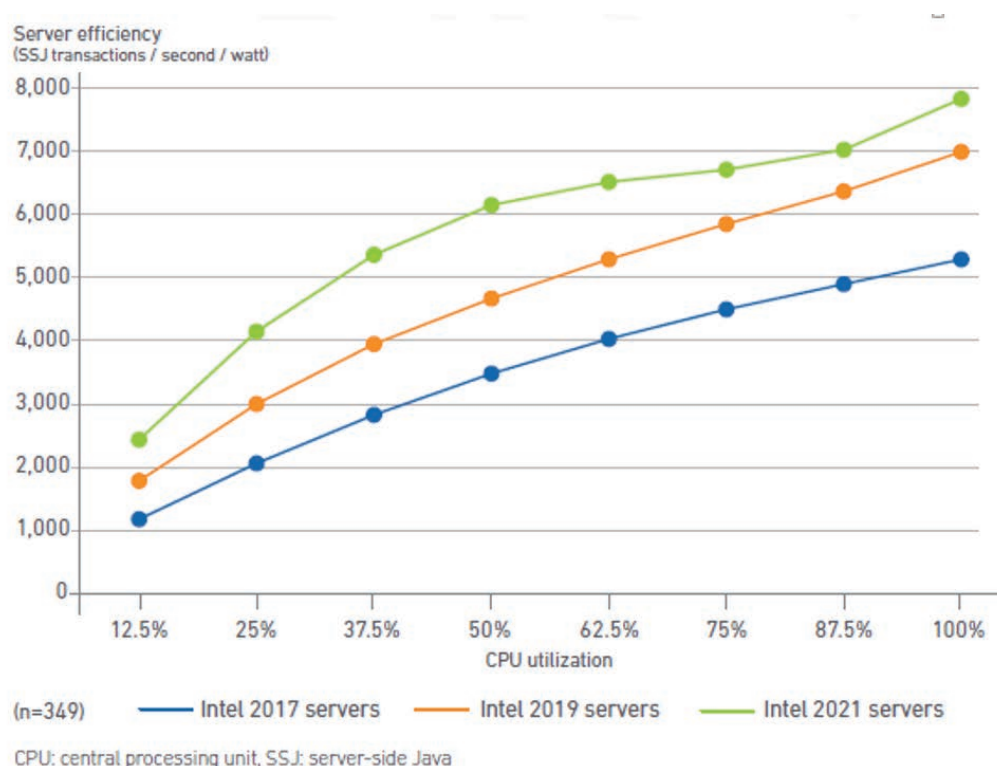
Figure 10: Server efficiency increased based on CPU utilization
