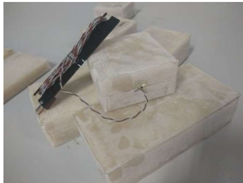
Picture 6. Standardized load packages, including an M-package with an embedded temperature sensor
