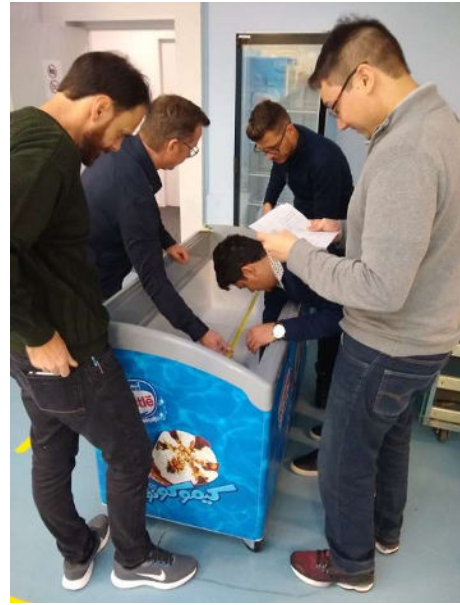
Picture 7. Practical session: Volume and total display area measurement exercise on ice-cream freezers
