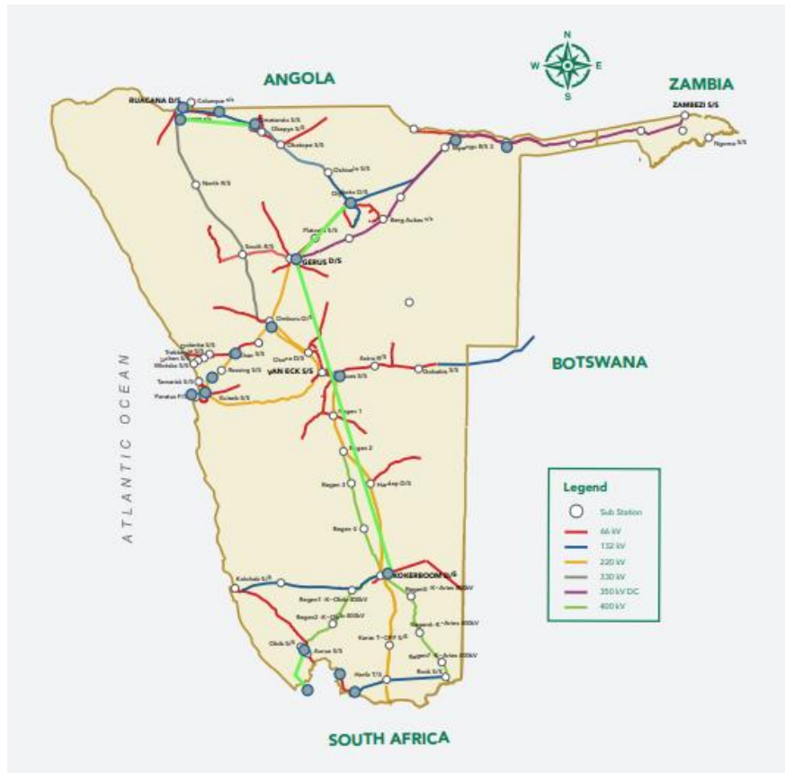
Figure 7-1: Generation and transmission network in Namibia. Image Source: Namibia: Geospatial Least Cost Electrification Plan, 2021
