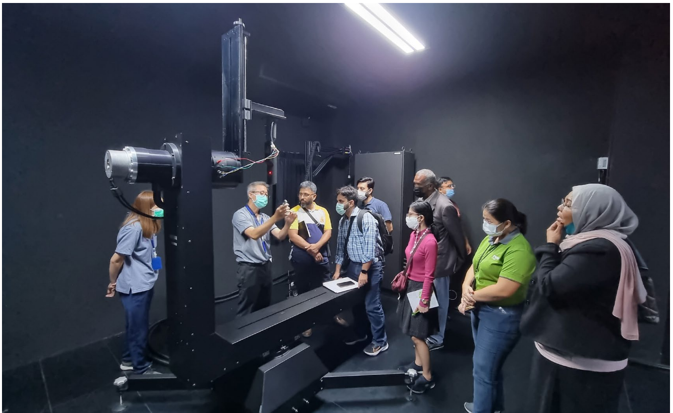
Picture 14. Observing testing of Pakistan streetlight in the rotating-source goniophotometer with C,y coordinate system. Discussion is on effects on test results of rotated operating position, stray light and dead angle
