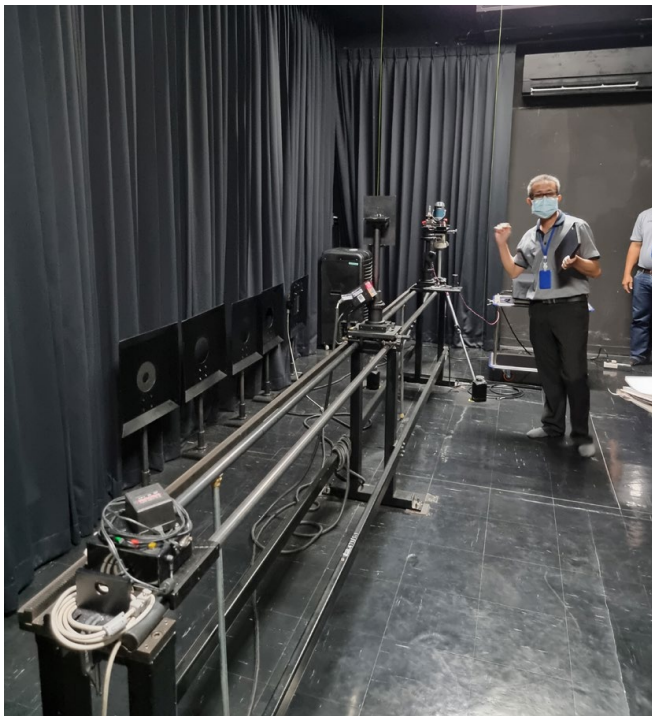
Picture 3. Inspection of optical bench used for calibration of reference light sources (for luminous intensity) as well as calibration of illuminance and luminance meters
