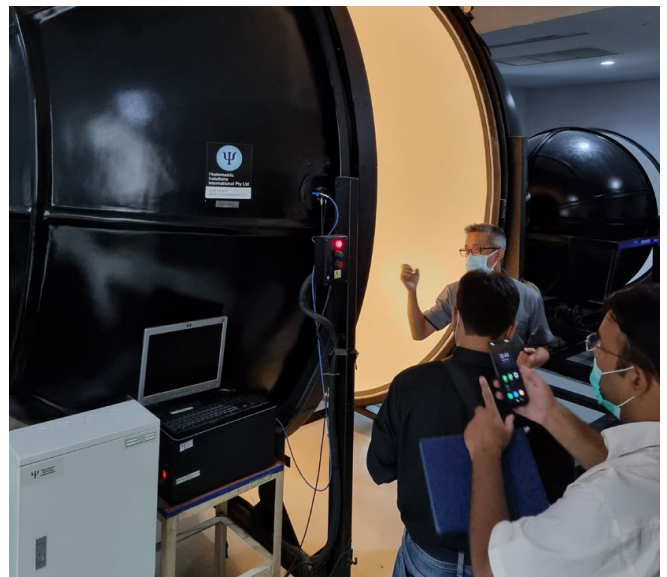
Picture 5. Inspection of 3 metre diameter integrating sphere, used for measuring total luminous flux and colour quantities of light sources ranging from small lamps to large luminaires
