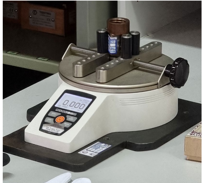
Picture 11. Inspection of a mechanical test for electrical safety of lamps: torsion test for secure fixing of lamp cap to the lamp
