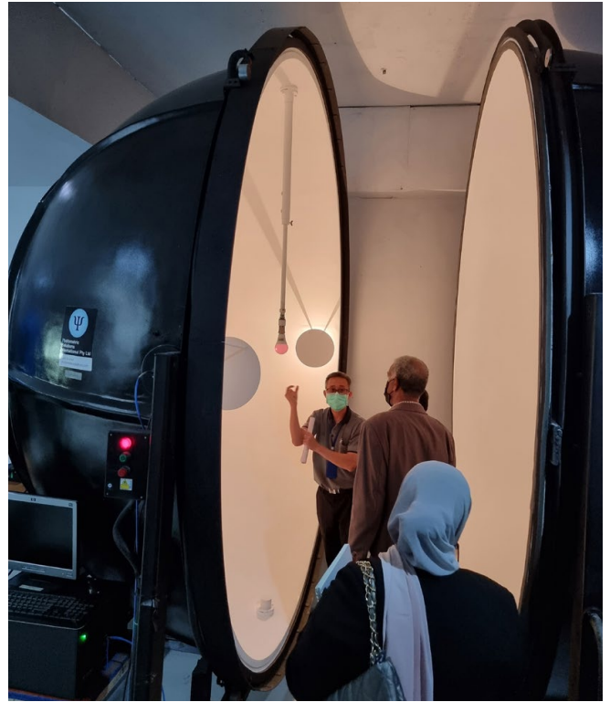
Picture 13. Observing testing of Pakistan lamp in integrating sphere. Discussion is on the positioning of the lamp at the optical centre of the sphere by use of a laser positioning system
