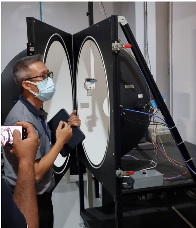
Picture 6. Inspection of 0.5 metre diameter integrating sphere, used for measurement of luminous flux and colour quantities of small lamps
