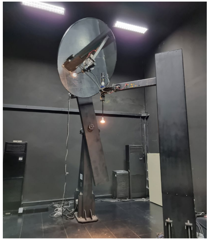
Picture 4. Inspection of mirror type goniophotometer with C, \gamma coordinate system, used for measuring luminous intensity distribution and total luminous flux of light sources
