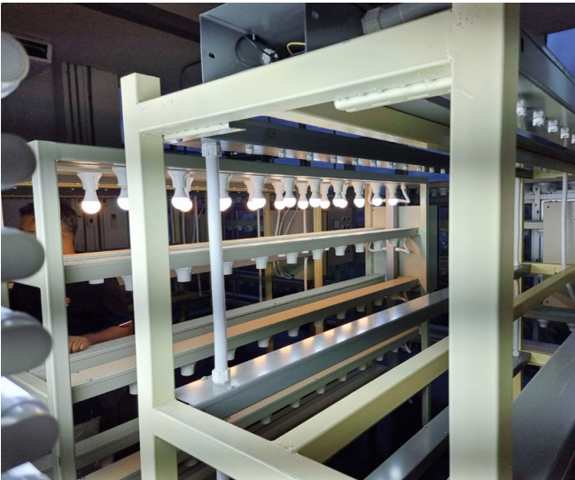
Picture 9 and Picture 10. Inspection of lamp and luminaire ageing facility, used for endurance testing and lifetime measurement (based on light loss over time). Can be used for pre-burning (warm up) of lighting products prior to photometric and colorimetric measurements
