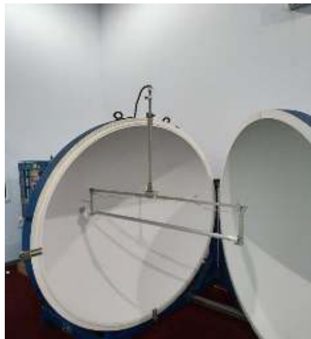
Figure-5. Sample Placement of Self-ballasted Tube LED
