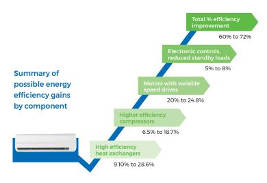
Various efficient technologies and components can improve the energy efficiency of air conditioners.
