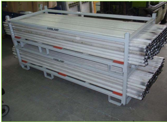
Container for fluorescents > than 2 metres
