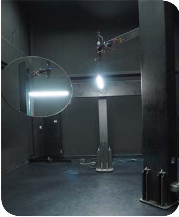
■ Goniophotometer at Electrical and Electronics Institute laboratory, Thailand (Photograph courtesy of Marie Leroy, UNEP)
