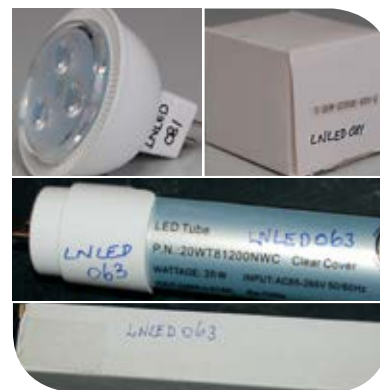
Figure 5 Examples of identification codes on a MR16 LED lamp and a linear LED lamp and their packaging
